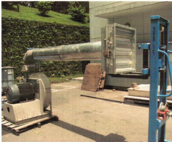
Figure 6 : Setup of "CCC-VCD 400" Volume Control Damper for Air Leakage Test
